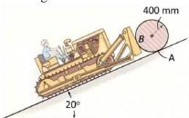
The coefficient of static friction between the dozer bucket and the spool (Point B) is 0.45, and coefficient of kinetic friction between road and the spool (Point A) is 0.15. Consider the spool only slides up the incline. The maximum normal force in N acting at Point B, is \_\_\_\_\_. (GATE 2023)
